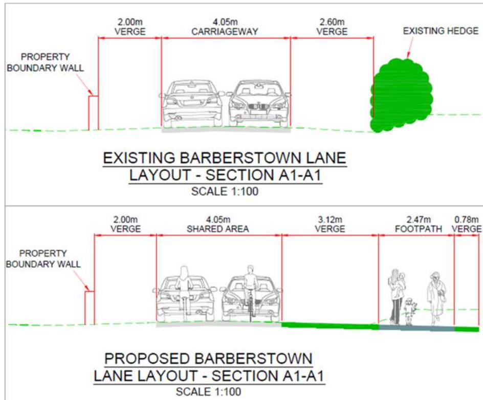
Figure 5.25 Existing and Proposed Cross Section Barberstown Lane North Access Road
